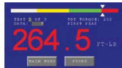
Example shows testing a 250 ft.lb. wrench at 100% of full scale. Red indicates high reading.
