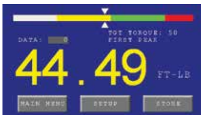
Example shows testing a 250 ft.lb. wrench at 20% of full scale. Yellow indicates low reading.
