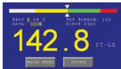
Example shows testing a 250 ft.lb. wrench at 60% of full scale. Yellow indicates low reading.
