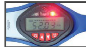
The red LED illuminates 4% beyond target torque, indicating fastener was overtorqued. Rapid "alarm" buzzer sounds.
