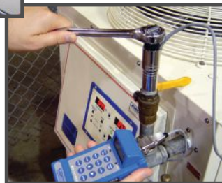
...into a highly accurate digital torque tool.
